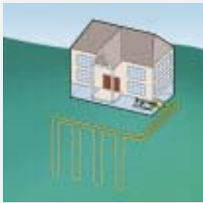
Vertical Closed Loop (Geothermal Consortium)
