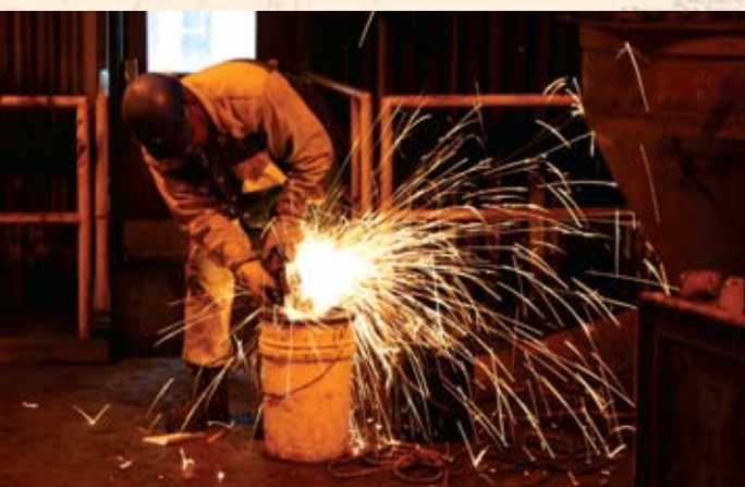
Mechanic I Charles Gray grinds a part while making repairs to a classifier
