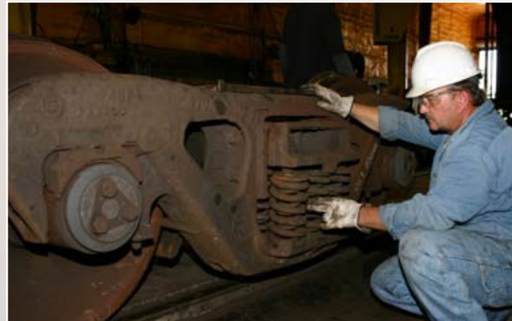
Mechanic Jerry Denson inspects the springs on a railcar truck assembly.
